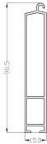
ALUMINIUM EXTRUDED GUIDE CHANNEL (90x35mm)
